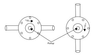
Connect appropriate connector from pick-up from DCS or electronics.
