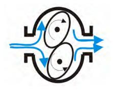
The flow through the meter measurement chamber follows the path of least resistance. Therefore no liquid passes through the center cavity between the rotors. The fluid is displaced from the inlet to the outlet via the area between the smooth oval rotors and the inner diameter of the meter housing.
