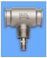
**Note:** Turbine meter should be installed in the vertical direction with flow direction up to ensure proper drainability.
