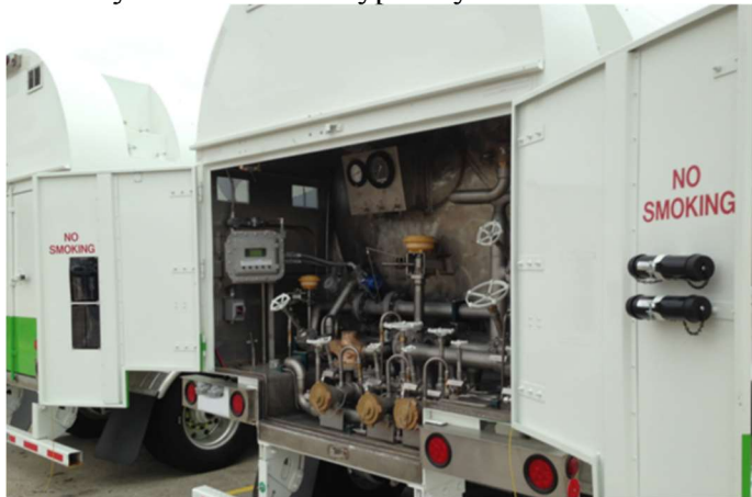
Hoffer Cryogenic Flow Measurement System installation shown above for measurement of LNG on road tankers.
