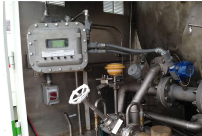
A closer view shows more detail of the Hoffer System which is typically installed in the rear of the tanker.
